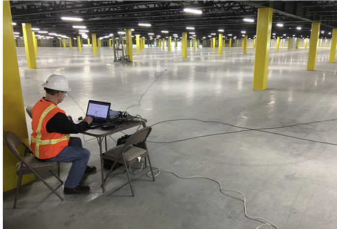
Dr. Brad Davis, University of Kentucky, measured floor vibration in a retail distribution center. Vibration testing confirmed the predicted results.
